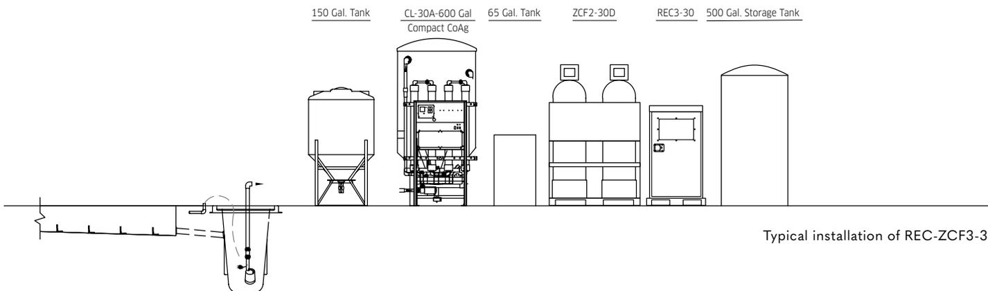
Typical installation of REC-ZCF3-30
